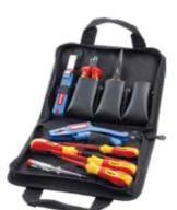
Contents: VDE tested 1000V insulated tools: Insulated Screwdriver 1000 V slotted: 3x100, 5,5x125 mm. Insulated screwdrivers 1000 v Phillips PH1, PH2. - 1 Insulated Diagonal Cutter 1000 V-160 mm.
